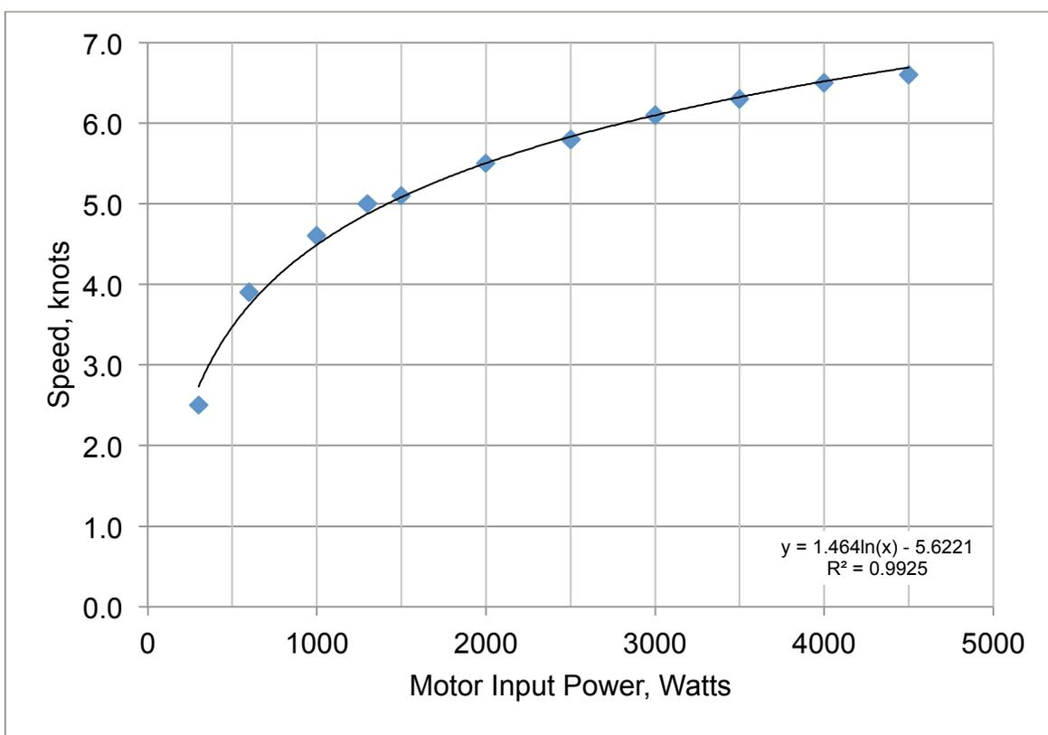
As you can see, Wayward Sun will go 4.5 knots at 1000 Watts and 5 knots at 1500 Watts. Doubling the power from 1500 Watts to 3000 Watts will gain just over an additional knot of speed. Add another 1500 Watts gets you only get another half knot to max out our top speed of 6.5 knots at 4500 Watts of power. For Wayward Sun, the sweet spot on the curve is around 4.5 knots. Notice that it takes only 300 Watts to move our boat at 2.5 knots.
