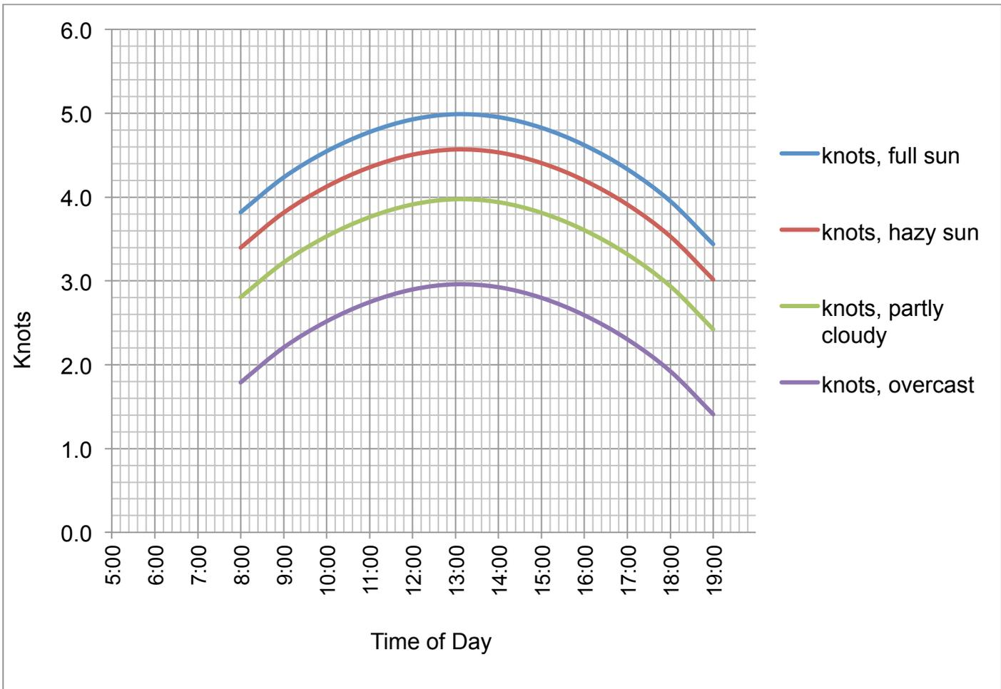
The second graph eliminates the power axis by mapping time of day directly to speed and so it's the solar cruiser's most direct way to predict their route for the day, or to plan a trip in advance.
